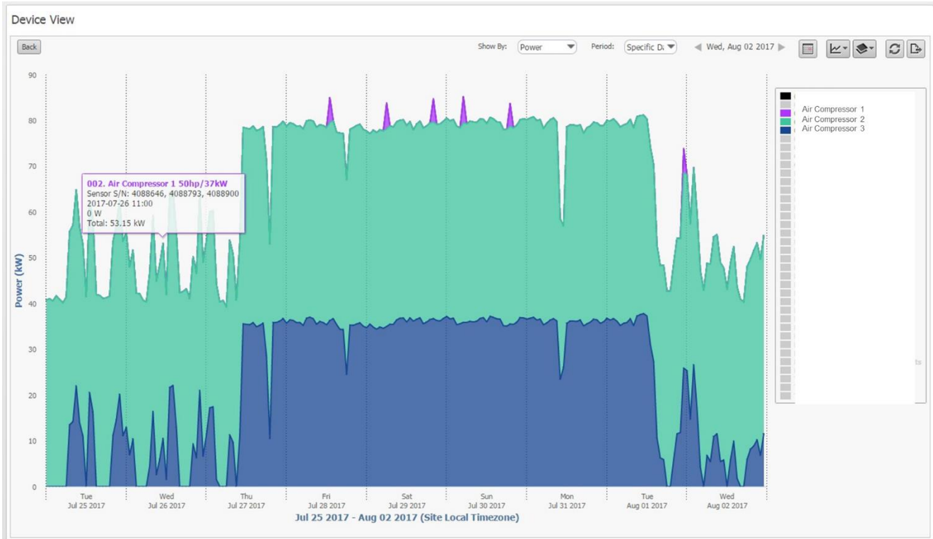
Figure 4. Site Air Compressors Daily Energy Usage Comparison, Device Level View
